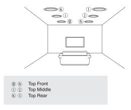
Ceiling speakers, etc. are used for maximizing effects in Dolby Atmos or Dolby Surround listening mode. Install Top Front speakers midway between the position just above the listening position and the position just above the front speakers. Install Top Middle speakers just above the listening position. Install Top Rear speakers midway between the position just above the listening position and the position just above the surround back speakers.
